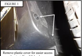
when installing M6 hardware.
