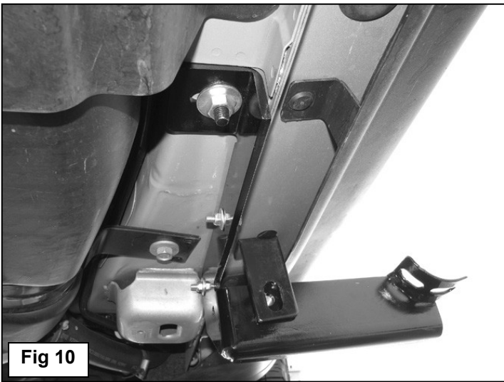
(Fig 8A) Driver side rear Mounting Bracket location
