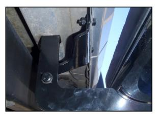
6. Repeat steps 3-5 for the driver rear mounting bracket and support bracket. Do not fully tighten at this time.
