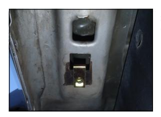
2. Starting at the front driver side mounting location. The bottom rocker mounting hole may be covered by black tape. After removal, insert an M8 clip nut through the square hole. Some vehicles may already be equipped with a threaded hole.
