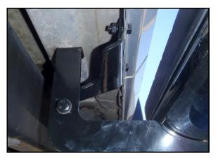
6. Repeat steps 3-5 for the driver center and rear mounting bracket and support bracket. Do not fully tighten at this time.
