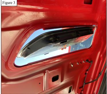
5. Locate the light pods. Using the supplied M4 Phillips bolts in the light box and the supplied M4 serrated flange nut (item 11), assemble the light to the hood scoop. Tighten the M4 hardware to 25 in-lbs. See Figure 4. Note: Disregard the extra M4 hex nut in the light box as it is not needed.
