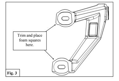
6. Place foam squares on the underside of each cowl mount foot and trim as necessary. See **Figure 3**.
