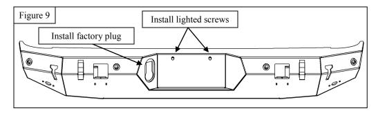
12. Adjust bumper as necessary and torque down all hardware to specified ft-lbs: M4 to 2 ft-lbs, M6 to 7 ft-lbs, M10 to 35-40 ft-lbs.
