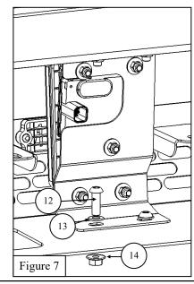
9. Use the supplied M8 Hardware (Items 12-14) to attach the LED Brackets (Item 4) to the center section. See Figure 8.
