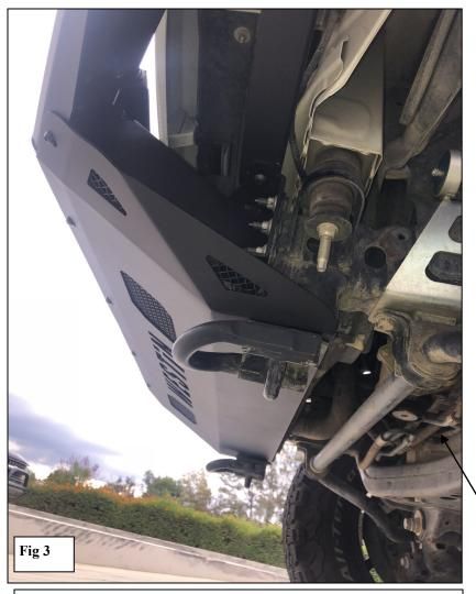
Remove factory tow hooks, then attach skid plate. Then re-attach factory tow hooks using supplied M12 hardware or OEM hardware.
