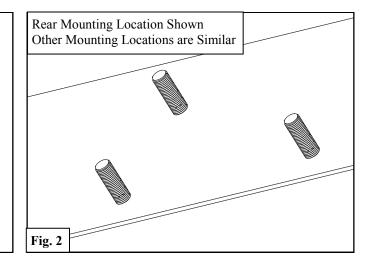
4. At the rear mounting location, loosely install Rear Mounting Bracket (6) with preassembled Universal Bracket (7) using the supplied M8 hardware. See **Figures 3 & 4**.
