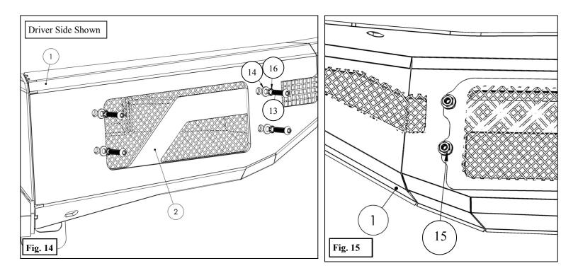
13. Align bumper as desired and torque all hardware as specified: M6 to 7 ft-lbs, M8 to 18 ft-lbs, M10 to 38 ft-lbs, M12 to 60 ft-lbs.
