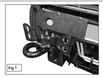
5. Remove the passenger/right side tow hook from the end of the frame, (Figure 7). Next, remove the (4) factory hex nuts, lower frame extension and double bolt plates from the end of the frame, (Figures 2 & 7). Repeat for Driver Side.
