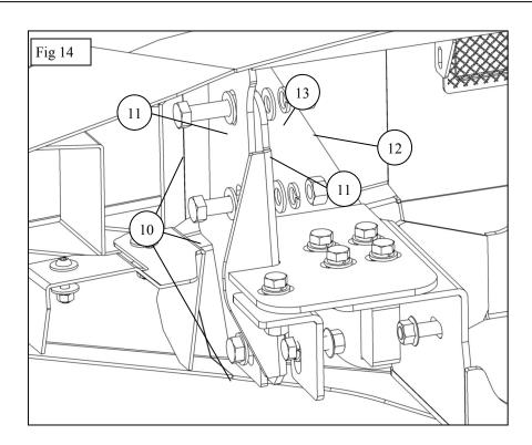
13. Adjust the bumper as needed and torque hardware as specified: M6 to 5-7 ft-lbs, M12 to 50-55 ft-lbs, M14 to 90-95 ft-lbs
