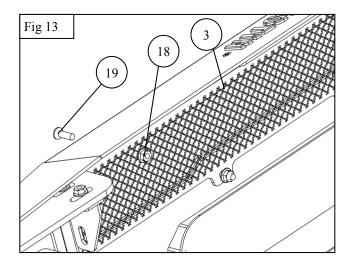
12. Using supplied M14 bolts, loosely assemble the bumper to the mounting brackets. See Figure 13
