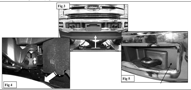
4. Place blocks or jack stands under the front bumper to support it during mounting bolt removal. Once the bumper has been safely supported, remove the (8) factory bumper bolts, (**Figure 6**).
