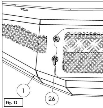
12. Align bumper as desired and torque all hardware as specified: M6 to 7 ft-lbs, M10 to 38 ft-lbs, M12 to 60 ft-lbs.
