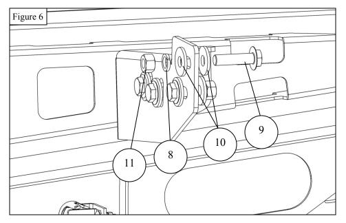
Insert the supplied M12 bolt plates into the bumper. See Figure 7.
