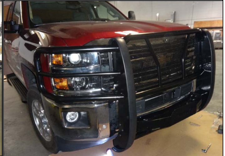
HDX Winch GG Installation Complete
