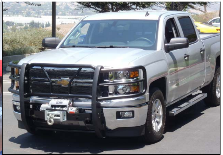
HDX Winch GG Installation Complete
