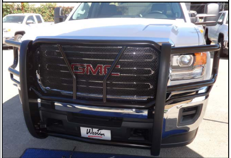
HDX GRILLE GUARD, INSTALLATION COMPLETE
