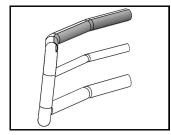
On polished grille guards. Anti-reflective tape is included to help reduce the amount of glare reflected from the headlights. It should be applied on the top tube section of the grille guard wings as shown on the illustration. Tape may need to be cut to correct length.
