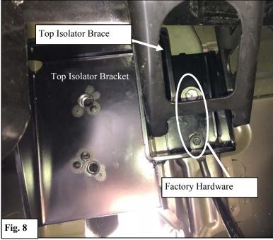
Driver Side Shown for 5.5 ft. bed. Top Isolator Bracket and Brace will be switched between driver and passenger side for 6.5 ft. bed applications.
