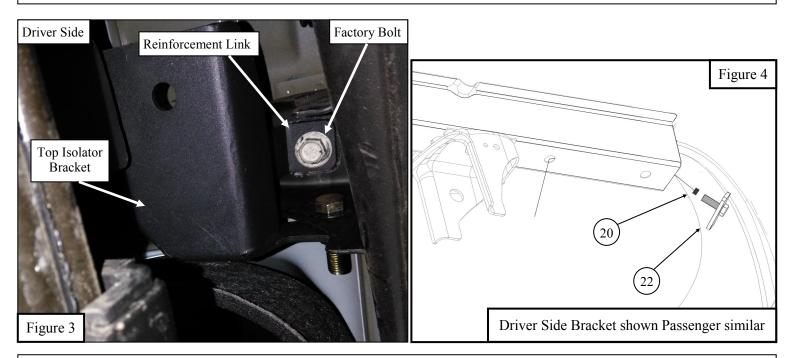
8. Attach the Bottom Isolator Bracket (5) to the Top Isolator Bracket (4) using the Isolator Kit (7) and hardware. See Figure 4.
