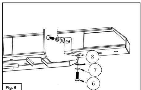
5. Align and adjust the step bars and brackets as needed, then fully tighten all hardware: M8 to 18 ft-lbs, M10 to 38 ft-lbs.
