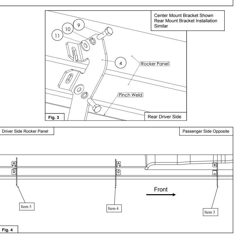
5. Mount the running boards on both sides using supplied M8 Hardware. See Figure 5 Note: All brackets mount to the running board/ drop step in the same way.
