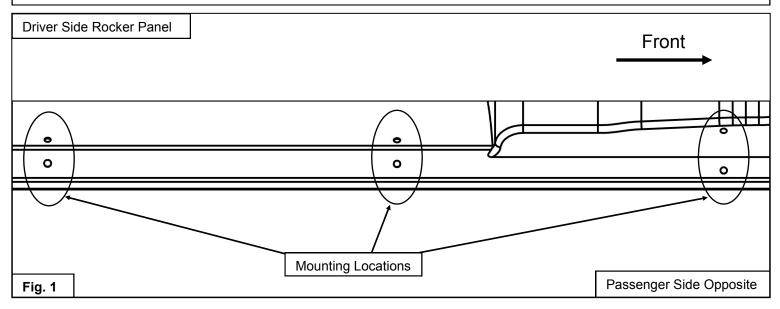
3. Loosely secure (1) Front Mount Bracket (item 3) to the rocker panel using the supplied M10 hardware . See Figures 1 & 2.
