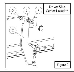
5. Locate (1) Center Mount Bracket (Item 2-3). Loosely secure Center Mount Bracket to the rocker panel using (2) M8 hex head bolt (2) M8 flat washer, and (2) M8 lock washer. See **Figure 2.** Refer to **Page 3** bracket orientation figures.
