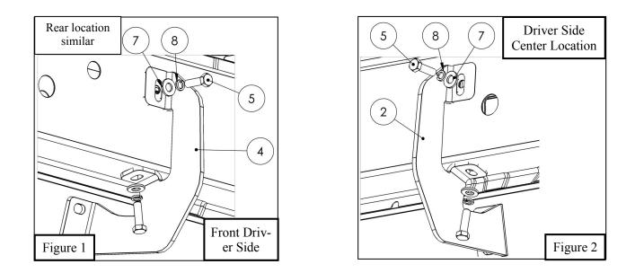
5. Locate (1) Center Mount Bracket (Item 2-3). Loosely secure Center Mount Bracket to the rocker panel using (2) M8 hex head bolt long, (2) M8 flat washer, and (2) M8 lock washer. See **Figure 2.** Refer to **Page 3** bracket orientation figures.
