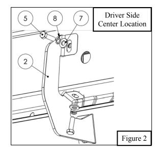
5. Locate (1) Center Mount Bracket (Item 2-3). Loosely secure Center Mount Bracket to the rocker panel using (2) M8 hex head bolt long, (2) M8 flat washer, and (2) M8 lock washer. See **Figure 2.** Refer to **Page 3** bracket orientation figures.
