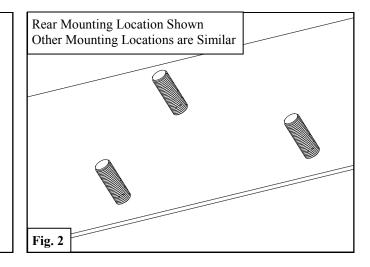
4. At the rear mounting location, loosely install Rear Mounting Bracket (6) with preassembled Universal Bracket (5) using the supplied M8 hardware. See **Figures 3 & 4**.
