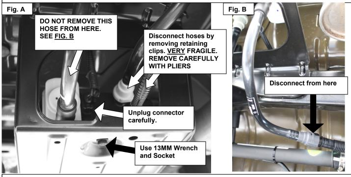
3.Proceed to remove the evap canister from the stock skid plate by removing the bolt at the bottom using 13MM wrench and socket. See Fig. A
