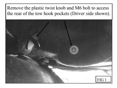
3. **Vehicles with factory tow hooks:** Remove the tow hooks by unscrewing the small bolts from the front of the hook and the large nut from the rear of the hook. Once the hook has been pulled through the front of the tow hook pocket the tow hook mounting bracket may be taken off by removing the two M10 bolts holding it in place. Refer to Figures 2 & 3. Note: The factory tow hooks cannot be re-used.
