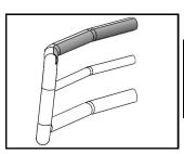
On polished grille guards. Anti-reflective tape is included to help reduce the amount of glare reflected from the headlights. It should be applied on the top tube section of the grille guard wings as shown on the illustration. Tape may need to be cut to correct length.
