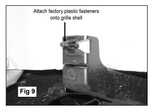
Titan & 04-07 Armada shown, without grille on for photo purposes. Note: Grille should be reinstalled before attaching Grille Guard
