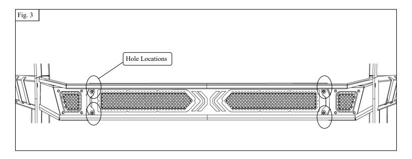
3. Adjust the Face Plate as needed for correct fitment. Torque Down all hardware to 4 ft/lbs.
