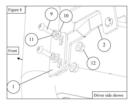
12. Align bull bar as necessary and torque hardware as specified: M10 to 40 ft-lbs, M12 to 60 ft-lbs. *Note: If you are installing the optional light bar, follow manufacturer's instructions.*
