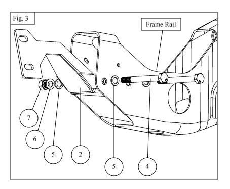
Using supplied M10 hardware, loosely assemble the bull bar on to the mounting brackets. See Figure 4.
