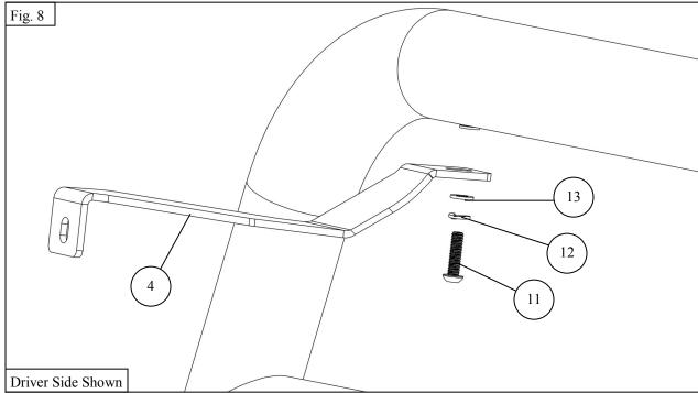
7. Adjust the bull bar as needed and torque all hardware as specified: M8 to 15-18 ft-lbs, M12 to 45-50 ft-lbs.
