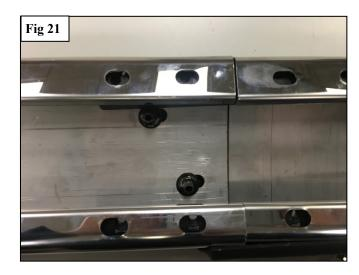
14. Obtain the Link Plate (5) and secure it to the Step Bar Assembly (1 & 2) using the supplied M6 Hardware. See Figure 22.
