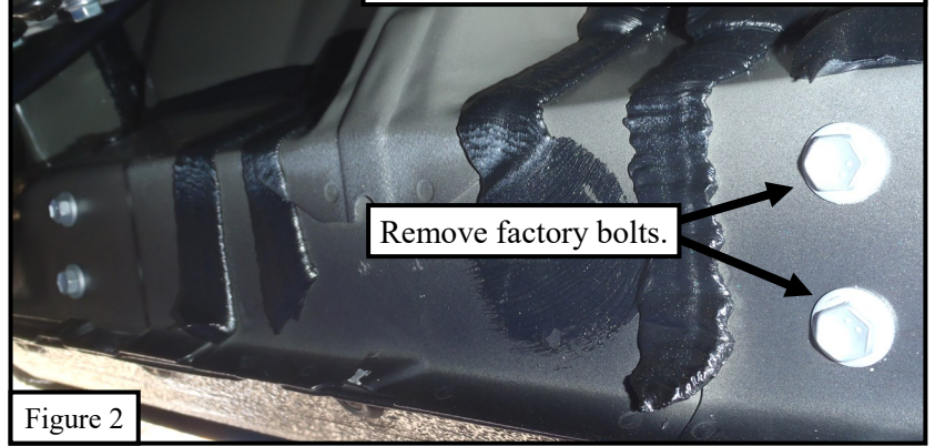
Center bracket rocker panel factory bolts.
