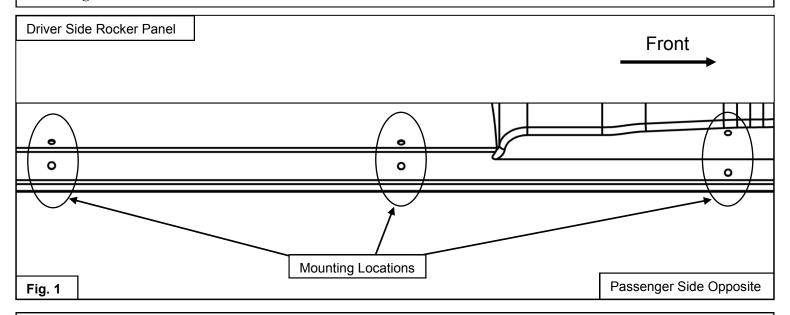
3. Loosely secure (1) Front Mount Bracket (item 3) to the rocker panel using the supplied M10 hardware . See **Figures 1 & 2**.
