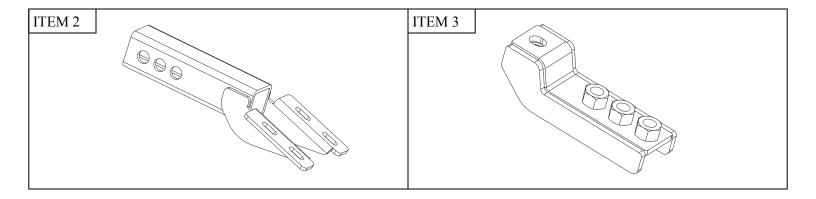
2. Loosely assemble the Anti-Rattle Bracket (3) to the hitch bracket (2) using the supplied M10 hardware. See Figure 1.
