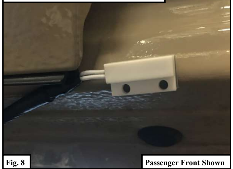
Place the Other Switch on the Edge of Rocker Panel Just Below the Door
