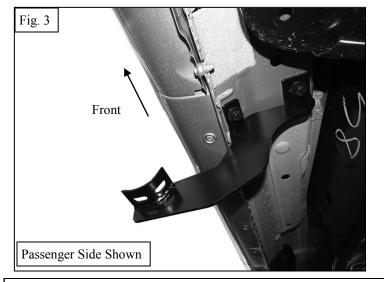
Locate the Center threaded mounting holes. Select (1) Center/Rear Mounting Bracket. Attach with (2) 10mm Hex Bolts,
