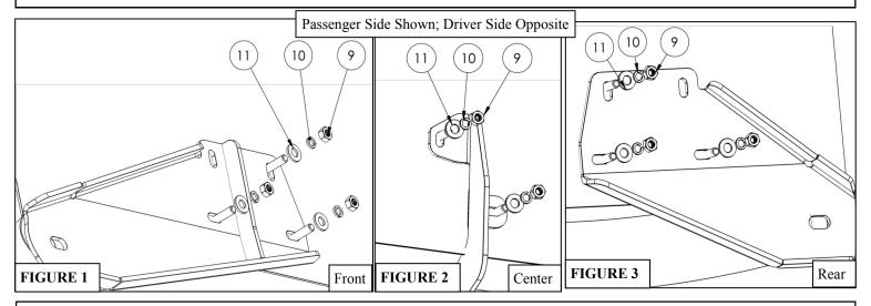
3. Loosely install the step bars onto the mounting brackets as shown in **FIGURE 4**. Note: The M10 rivet nut located on the bottom side of the step bar is approximately 2.0" biased toward the rear.
