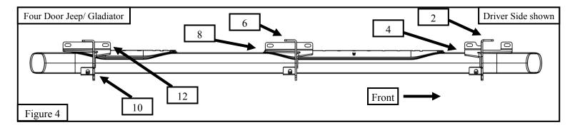
8. Align step bar and brackets to desired positioning then torque and tighten all: M8 hardware to 16 ft-lbs and M10 to 32 ft-lbs
