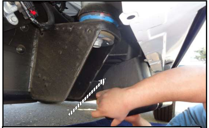
Remove the plastic cover by pulling it toward the side of the truck.
