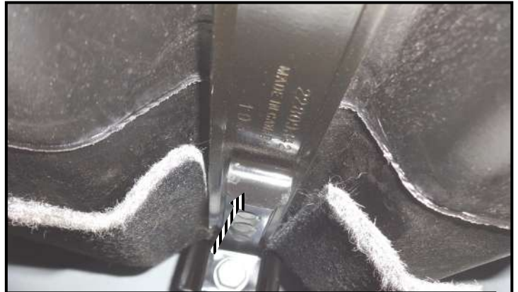
Using a ratchet with a long extension and a 13mm socket to loosen and remove the bolts of the tank support straps. Use an assistant to help hold the tank.
