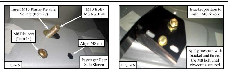
**FOR NEWER MODELS:** If the rocker panel has pre-installed M8 riv-certs or threaded holes, the M10 bolt / M8 nut plate will need to be positioned as shown in **Figure 8**.
