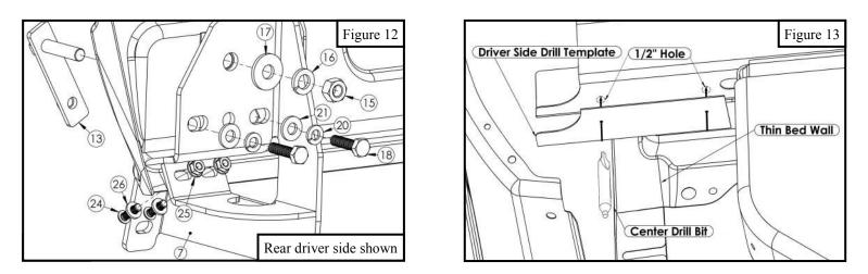
9. Locate (1) M10 fish wire (Item 28) and fish (1) M10 bolt / M8 nut plate (Item 13) through the rear drilled hole. Once bot bolt plates are placed, loosely install the Top Isolator Bracket (Item 11) with the supplied M10 hardware. (**Note:** Items 11 and 12 are identical). See **Figure 14**.
