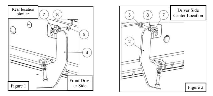
5. Locate (1) Center Mount Bracket (Item 2-3). Loosely secure Center Mount Bracket to the rocker panel using (2) M8 hex head bolt (2) M8 flat washer, and (2) M8 lock washer. See **Figure 2.** Refer to **Page 3** bracket orientation figures.
