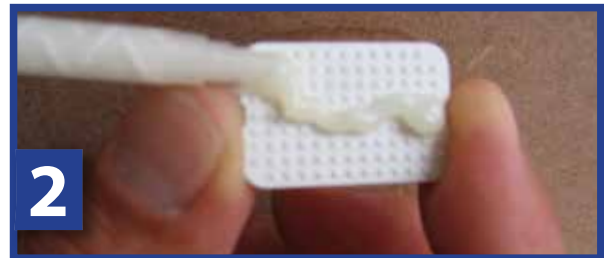
2 Squeeze the handle to dispense a small amount of adhesive onto the bottom of the part.
