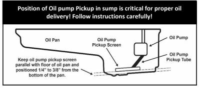
housing, this will provide a solid connection between the pump and pickup tube to prevent separation during severe use or vibration.
