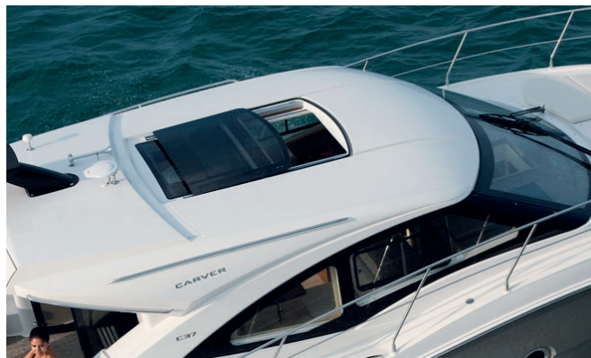
Standard electric marine sliding sunroof
