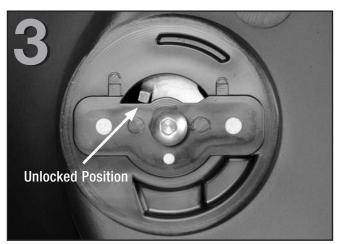
Identify the driver's side MudFlap by locating the "LH" mark located centrally in the recessed cavity on the tire side of the MudFlap. Ensure that the QuickTurn™ fasteners are in the fully unlocked position using the Allen wrench provided.
