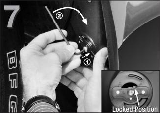
First ensure that the QuickTurn™ fastener is positioned properly by pressing in the direction indicated by arrow 1. Then, hand tighten the QuickTurn™ fastener (arrow 2). Verify that the QuickTurn™ fastener is in the fully locked position.
