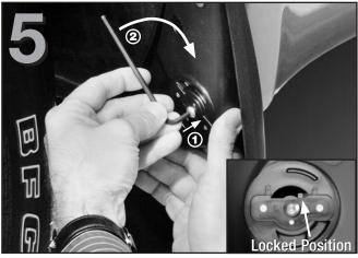
First ensure that the QuickTurn™ fasteners are positioned properly by pressing in the direction indicated by arrow 1. Then, hand tighten the bottom QuickTurn™ fastener (arrow 2). Verify that this QuickTurn™ fastener is in the fully locked position.
