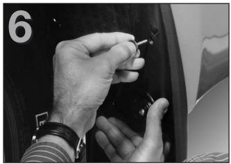
Press the MudFlap against the fender for a tight fit. Insert and snug the hex-head screw removed in step 3. **IMPORTANT** - Do not fully tighten at this time.
