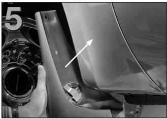
Position the smooth surfaced portion of the MudFlap so that it contours firmly against the fender as shown. **IMPORTANT** - Ensure that the QuickTurn™ fastener remains in the fully unlocked position during this step.
