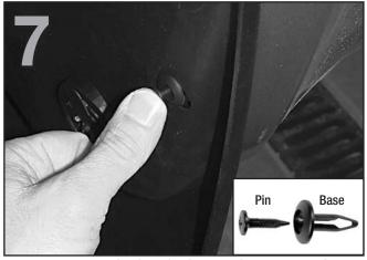
Prepare the plastic rivet for installation by removing the pin from the base. Insert the base fully into the top hole of the MudFlap and through the existing hole in the vehicle. Insert the pin into the base and press firmly to secure the rivet.
