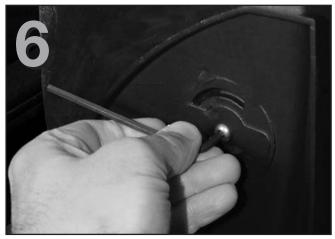
Repeat this process with the top QuickTurn<sup>™</sup> fastener.
