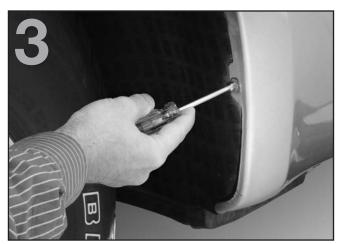
Remove the hex-head screw located in the position indicated in the photo. Do not lose this screw, as you will need it to complete the MudFlap installation.
