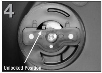
Identify the driver's side MudFlap by locating the "LH" mark located centrally in the recessed cavity on the tire side of the MudFlap. Ensure that the QuickTurn™ fastener is in the fully unlocked position using the Allen wrench provided.
